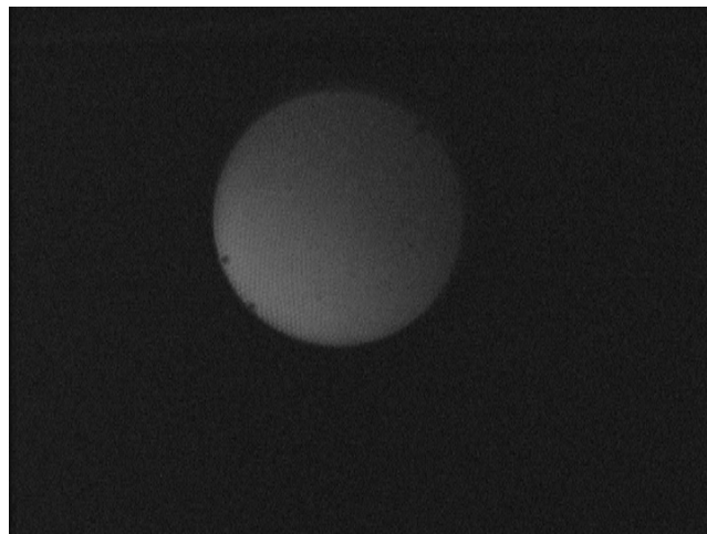
Figure 7a. Cross-sectional view of liquid R-134a in a capillary tube.
