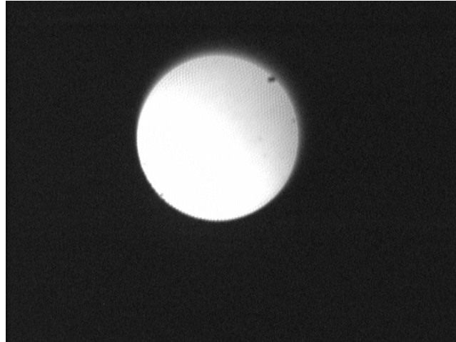
Figure 7b. Cross-sectional view of two-phase flow of R-134a in a capillary tube. The brighter area depicts the vapor phase.
