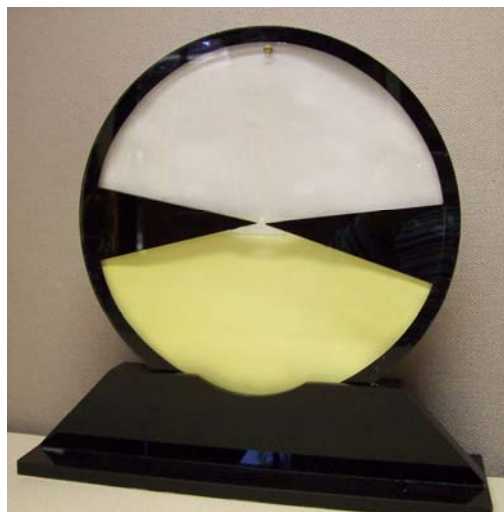
Figure 11 – Modified HSC with one gap in partition and stand. Note the small cork on the top.
