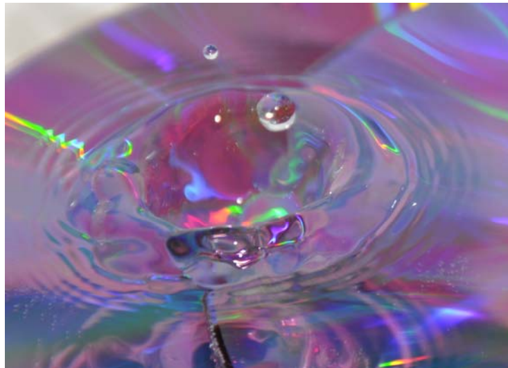
Figure 8 – Water drop impinging on a shallow pool of water over a CD.
