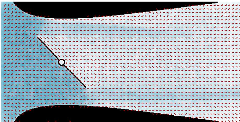
**Figure 8:** Uniform flow through a throttle valve. The mass density representation is superimposed by arrows illustrating the velocity field.<sup>13</sup>
