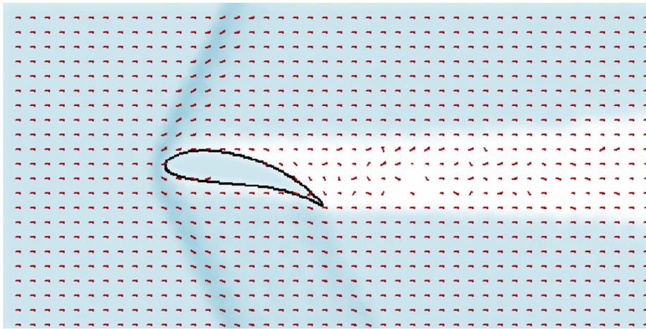
**Figure 7:** Uniform flow past a four-digit NACA airfoil. The mass density representation is superimposed by arrows illustrating the velocity field.<sup>13</sup>
