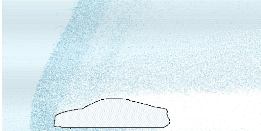
**Figure 5:** Uniform flow past a vehicle's contour. Mass density representation.<sup>13</sup>
