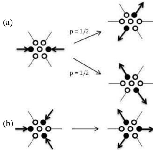
**Figure 2:** Collision rules for the FHP-I model, reduced by symmetry. Filled circles denote occupied cells and open circles empty cells. In-states are shown on the left hand side, out-states on the right hand side.
