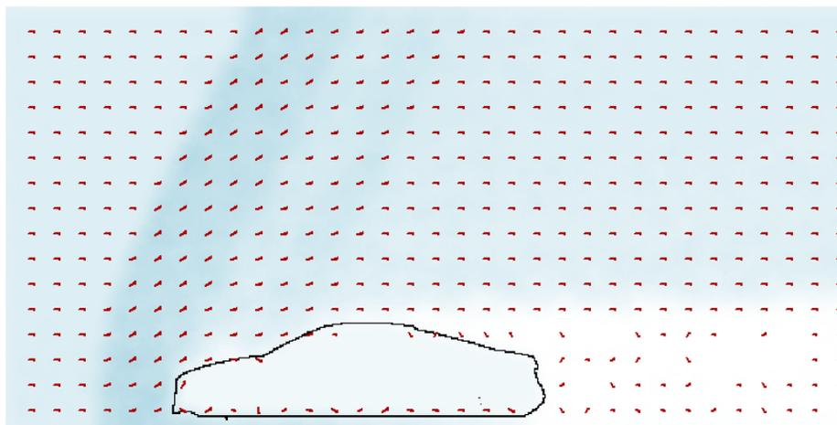
**Figure 6:** Uniform flow past a vehicle's contour. The mass density representation is superimposed by arrows illustrating the velocity field.<sup>13</sup>
