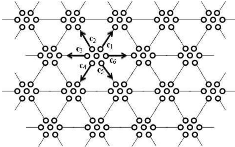
**Figure 1:** The triangular lattice of the FHP model shows hexagonal symmetry. The lattice velocities  $\mathbf{c}_i$  are represented by arrows. The circles at each node represent the seven channels corresponding to particles moving along the six directions of the triangular lattice and to the rest particle (center) in FHP-II.
