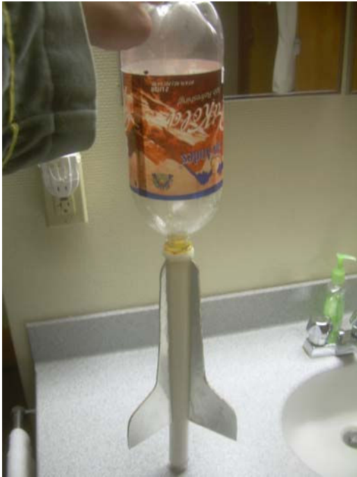
This rocket utilizes an extended nozzle system in an attempt to optimize thrust.
