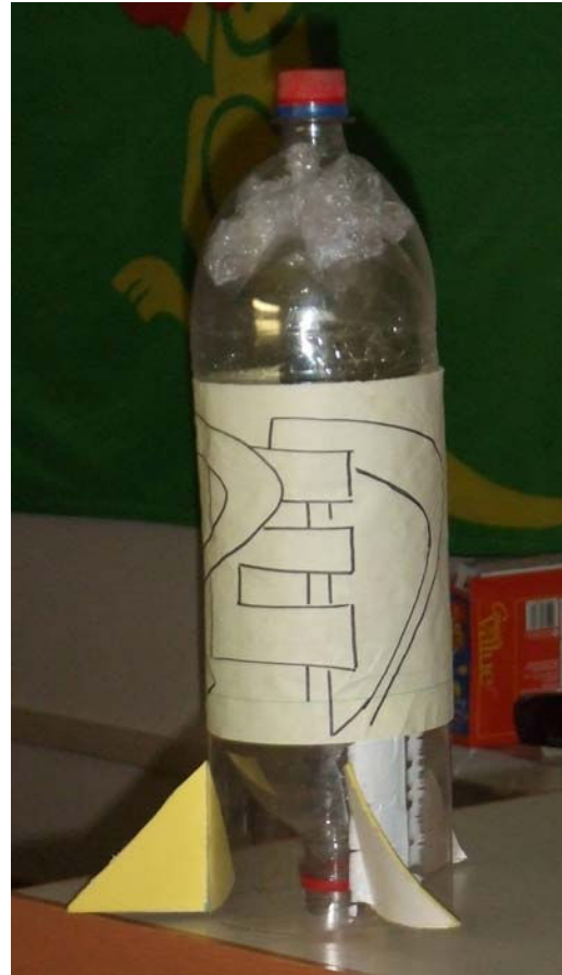
Curved fins on this rocket prototype are designed to increase stability by inducing spin, a concept introduced during the ME450 Stability Lab
