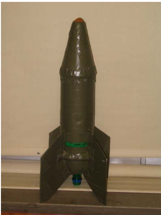
Durability was the primary objective of this sturdily built rocket. Large fins, coupled with a front-loaded center of gravity, created a large restoring moment to ensure stability in flight.
