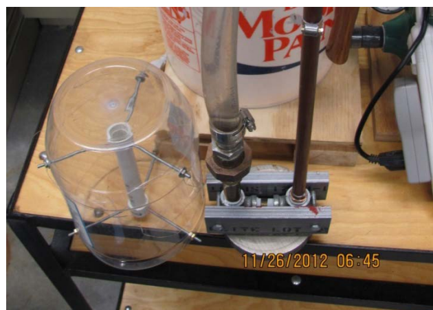
Figure 3. Photograph of the Jet Piping
