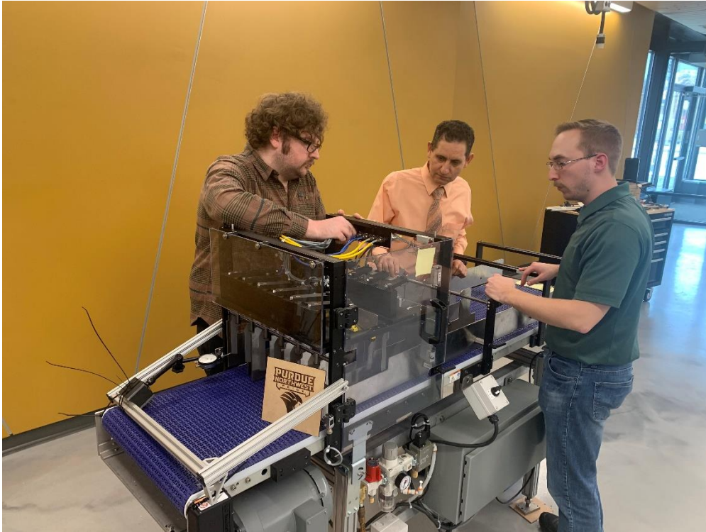
Fig. 4. Students discussing solutions for an adjustable escapement assembly.
