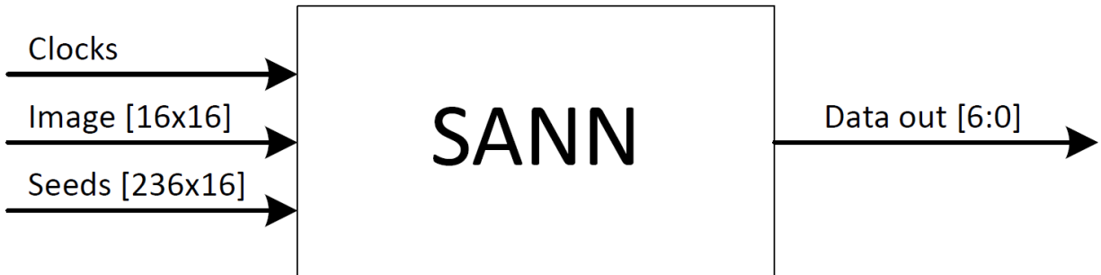
Figure 1. Overview of the SANN Interface. The SANN takes in the proper clocks, fixed seeds that are produced through training the network, and images (which the SANN will classify). The output of the SANN is a constantly running stochastic stream with values between -1 and 1.
