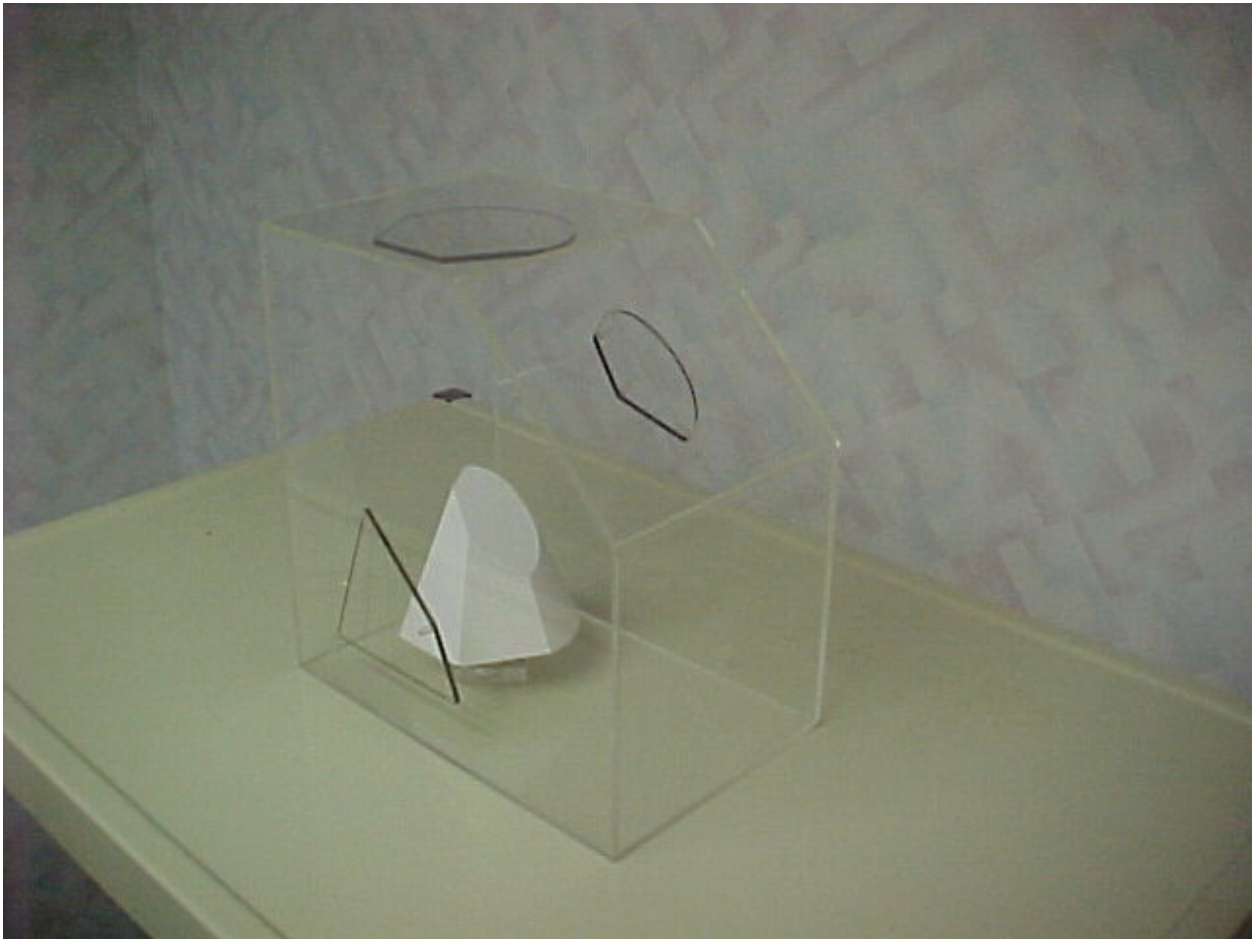
Figure 4 – Glass Box Used for Auxiliary Views
