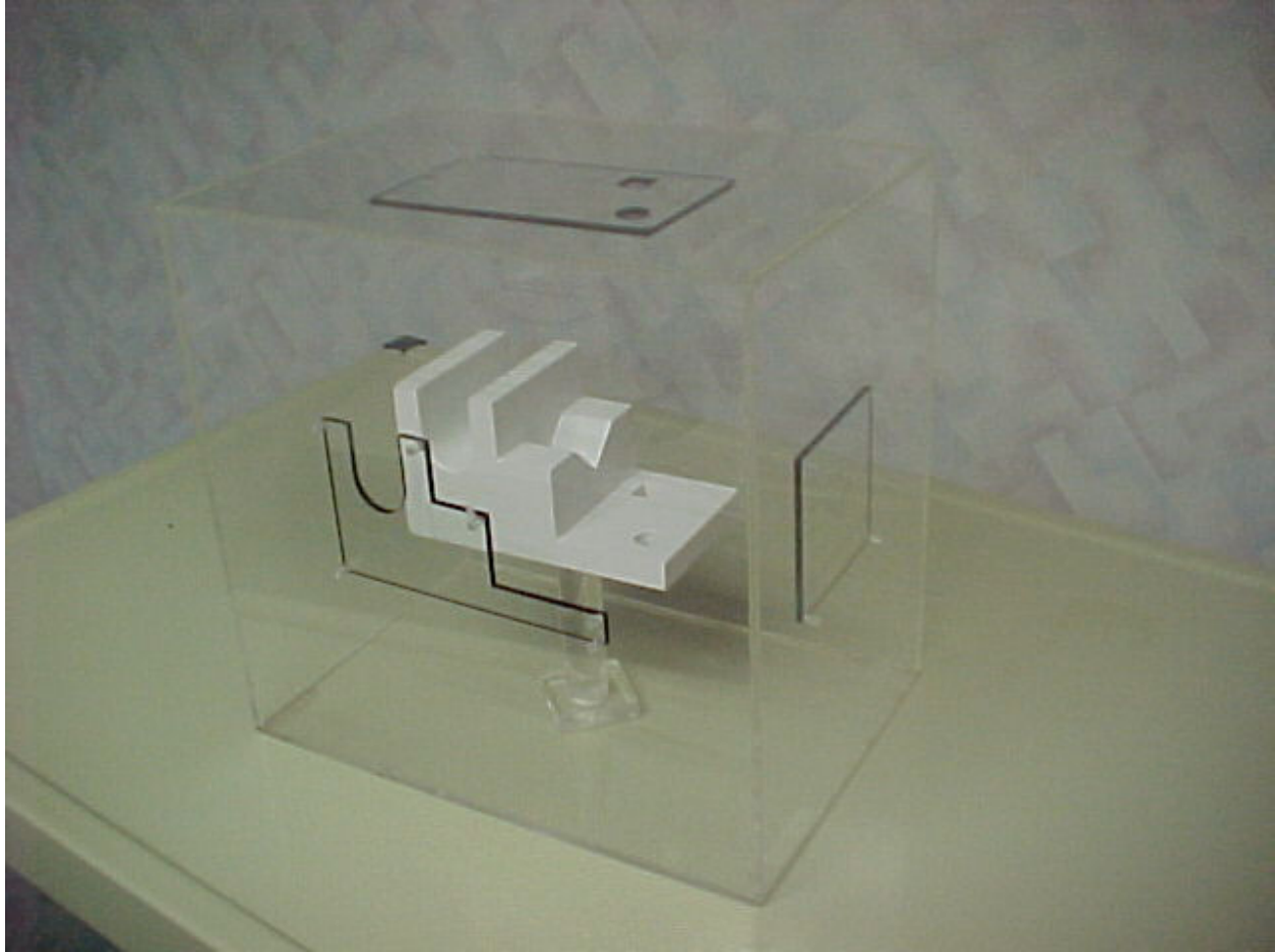
Figure 2- Glass Box for 3 View Drawings.
