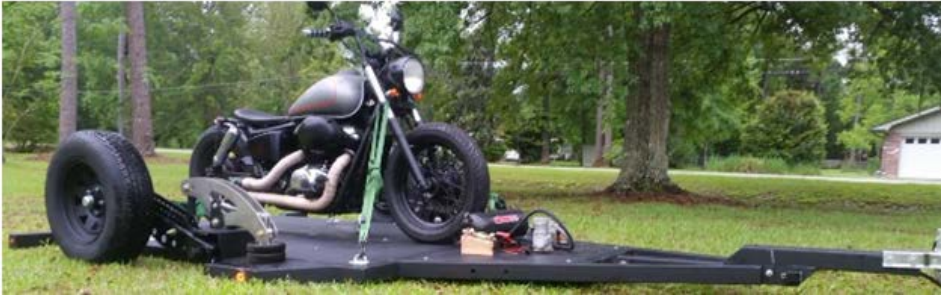
Figure 2 Final assembled trailer
