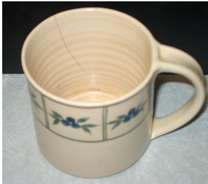
Figure 1. Crack revealed by coffee on the ceramic wall of a coffee cup
