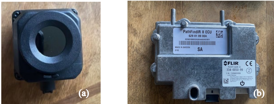
Fig 1. (a) FLIR PathFinder II IR camera; (b) The Electronic Control Unit (ECU).
