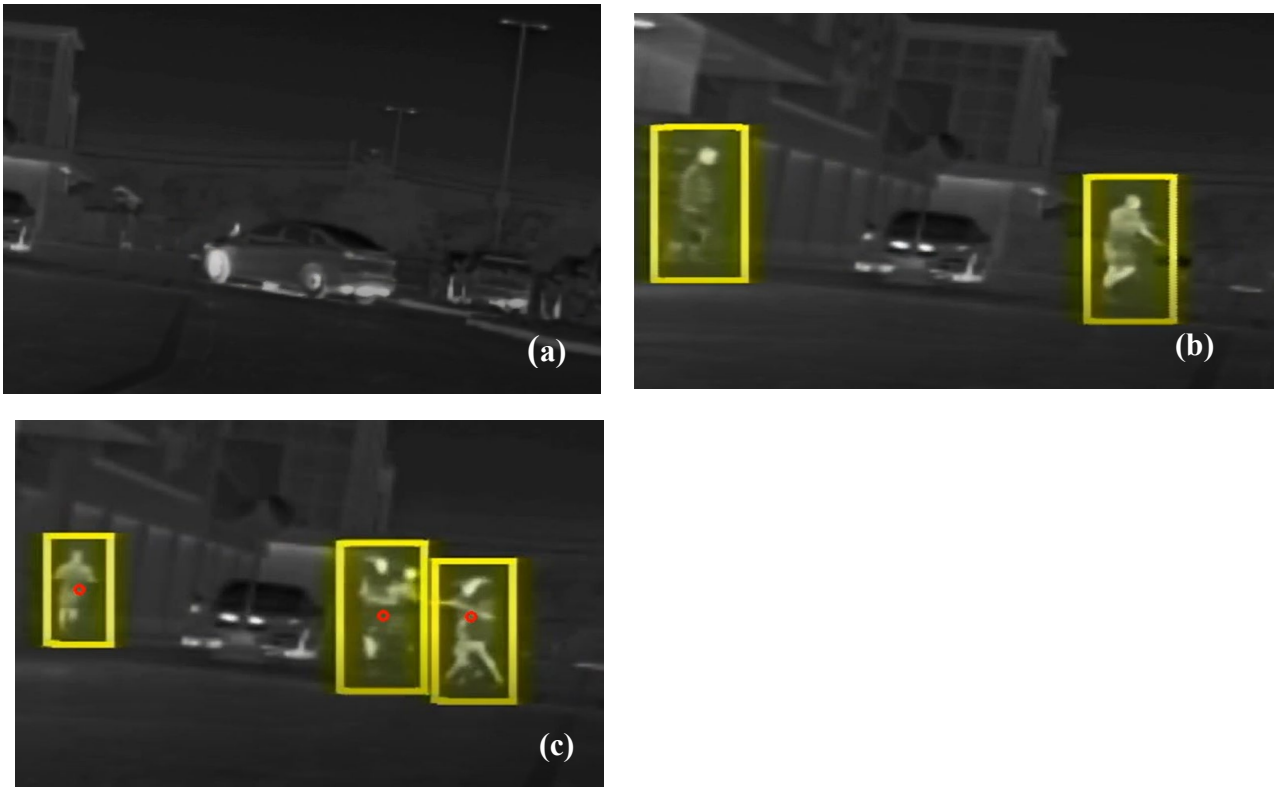
Fig.8 (a) Image capture without people or animals; (b) Two pedestrians are detected and labelled by yellow frames; (c) Centers of the yellow frames are marked out.
