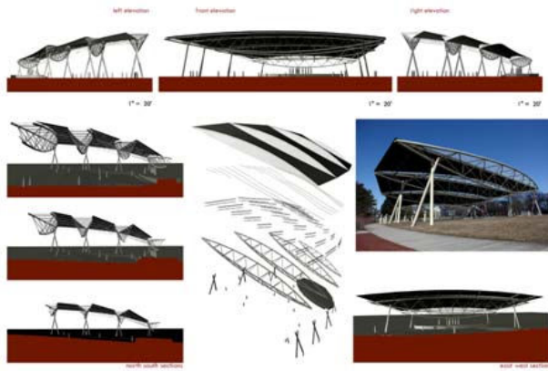
Figure 2a. Pavilion Design by Ryan Decker, Elevations (side views) and Sections (cut-away views).
