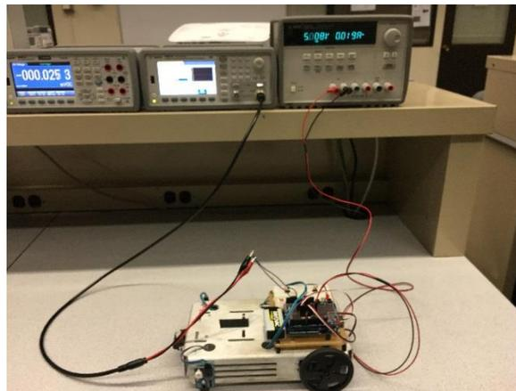
Figure 6. Hardware connection of autonomous vehicle
