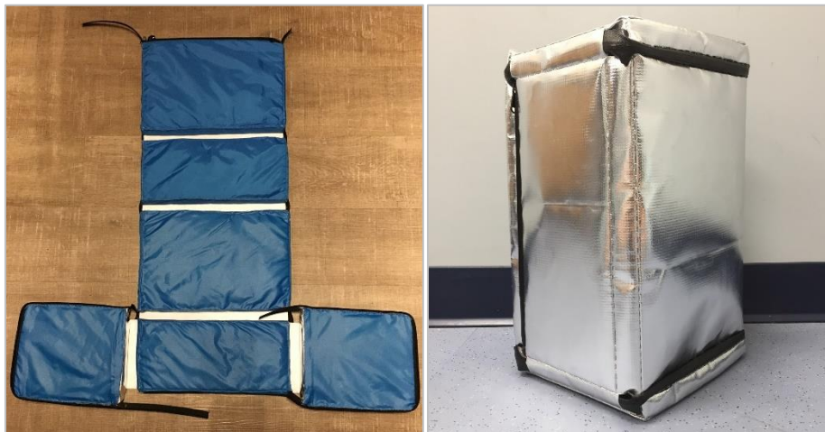
Figure 5: Photos that illustrate the completed scaled prototype Thermal Shield. The photo on the left depicts the Thermal Shield in its unzipped flattened orientation while the photo on the right shows the Thermal Shield assembled, zipped, and ready for shipment 3 .
