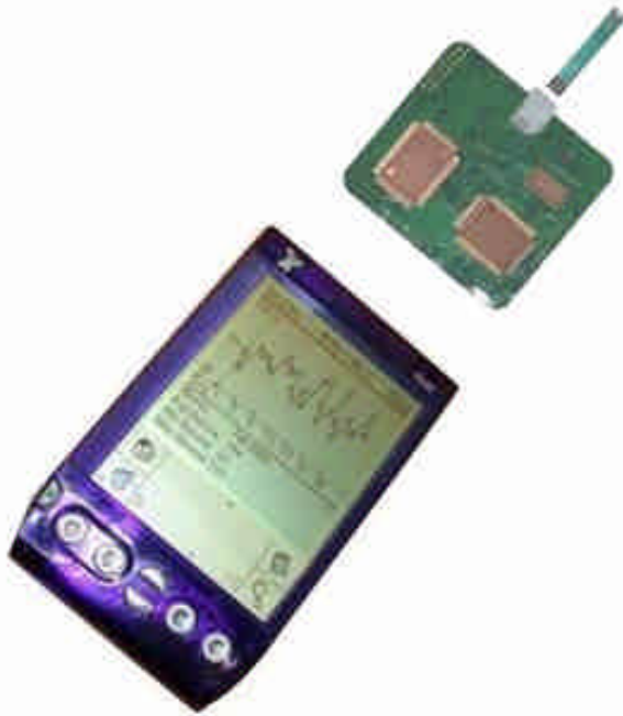
Figure 6. GlucoMon system showing software application, Springboard module, and test strip
