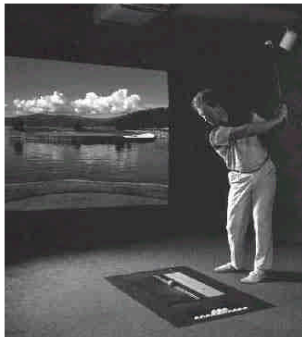
Figure 1 - Golf-Motion Measurement System. Note the floor-imbedded light sensors, golfer, and projected image on screen.
