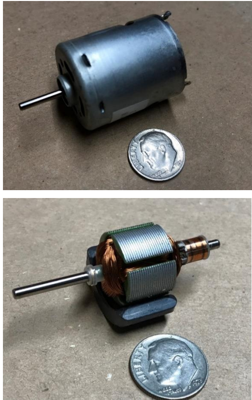
Fig.2: DC motor: Top) Assembled, and Bottom) Disassembled showing the wire coil attached to the motor shaft and one of two permanent magnets surrounding the wire coil.
