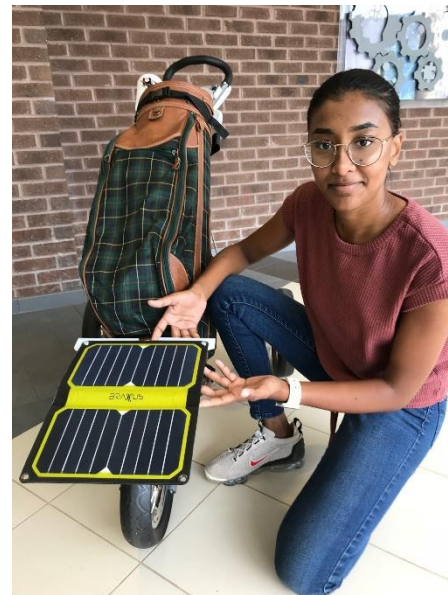
Fig 7: A solar panel was mounted to the front of the cart on a custom bracket.
