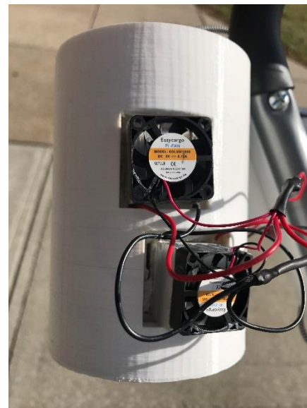
Fig 9: Top) The beverage holder showing the two wall design with thermal insulation between the walls. Also the curved copper plates are visible on the inside wall. Bottom) The two Peltier thermoelectric cooler assemblies viewed from outside the beverage holder.
