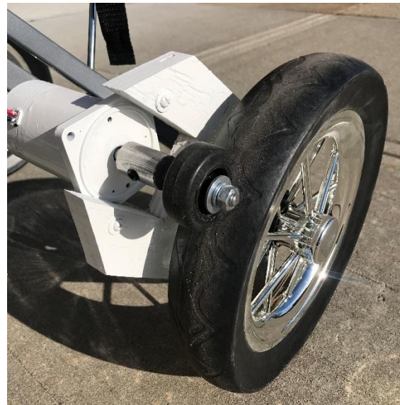
Fig 4: DC Motor “gear train” consisting of a small 2-inch diameter rubber wheel attached to the motor shaft and pressed against the surface of the 12-inch diameter golf cart wheel. The DC motor/generator is mounted behind the bracket.
