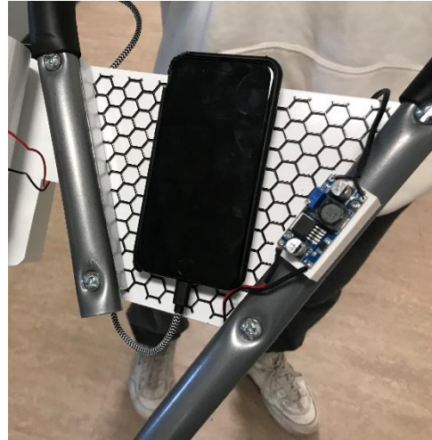
Fig 6: The cell phone mounted to the front of the golf cart panel. The panel was designed to be functional to support the attachment of the cell phone using a magnetic mount and to be aesthetically pleasing by using a decorative screen.
