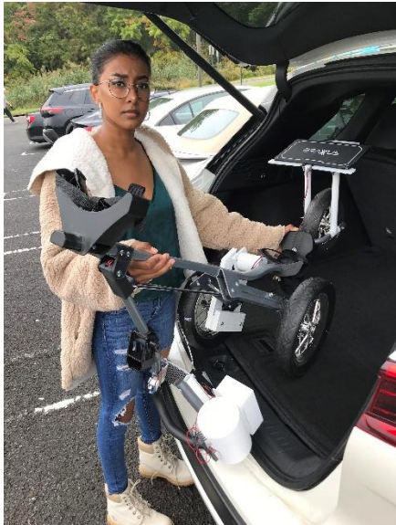
Fig 11: The golf cart was designed to maintain the easy foldability for transportation in an automobile trunk.
