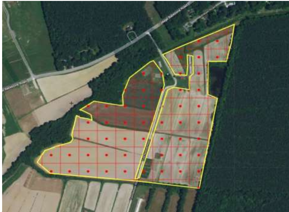
Figure 4. 2021 Soil Test Locations (Grid generated using Soil Test Pro)
