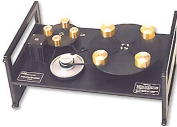
Figure 4: ECP 220 Industrial Emulator/Servo Trainer [3]
