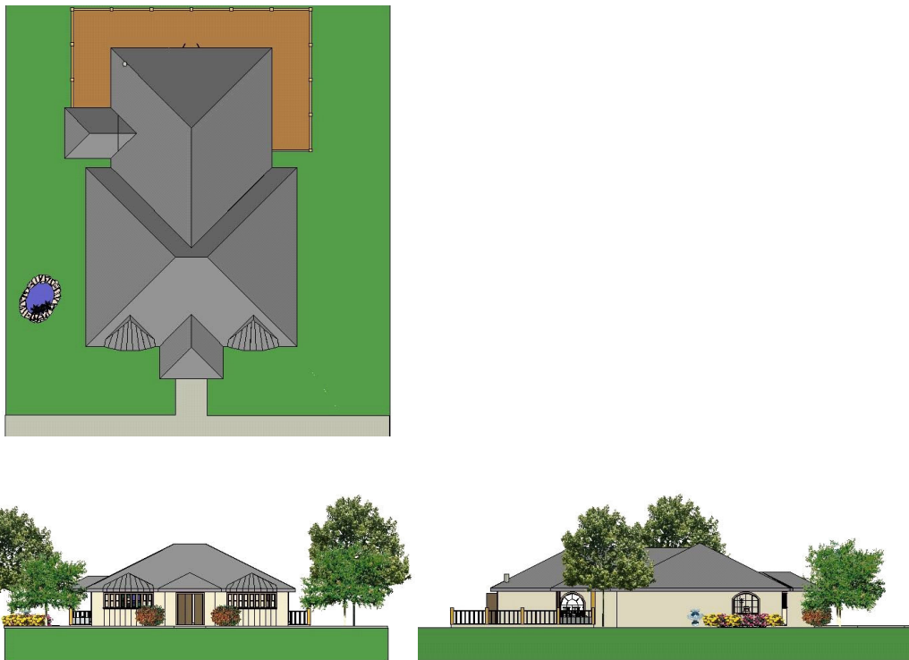
Figure 2. A Parallel, Third Angle Multi-view Student Elevation Submitted in Accordance with the Design Requirements for Phase 2, Project #1. 4
