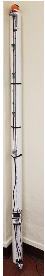
Figure 2: Falling Ball lab set-up
