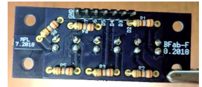
Figure 1: Back of PCB with resistors and pin header shown
