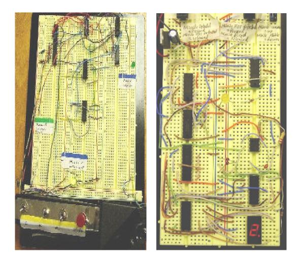
Figure 1. Typical projects 1 and 2. Students had the flexibility to include their own innovations, such as the seven segment display on the right.
