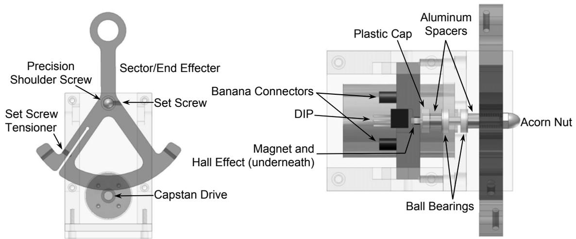
**Figure 3. Redesigned mechanical components of the Haptic Paddle**
