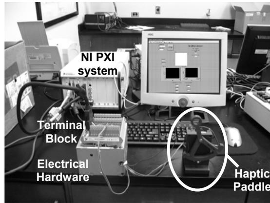
**Figure 1. The complete Haptic Paddle laboratory hardware system.**
