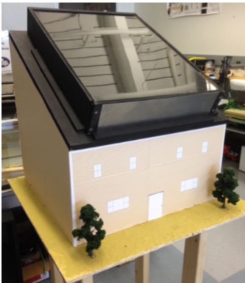
Figure 5: Testing unit with the plated collector placed on top.
