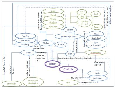
Figure 3. Detailed concept map for rotor, blades, hub, and controls.
