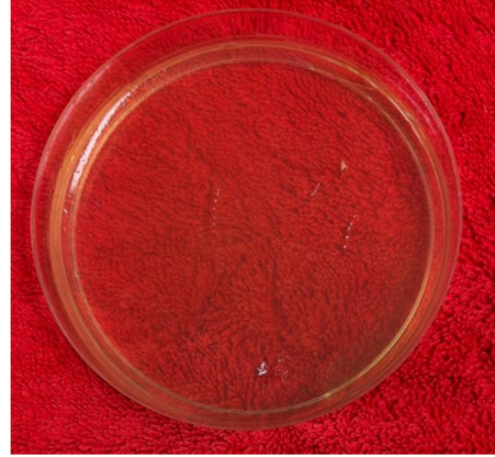
Figure 3 (b) The filtered well water which shows only 2 bacteria growth spots
