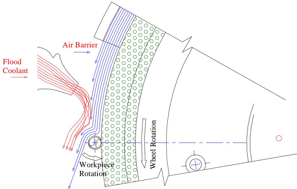
Figure 4: Illustration of Process with Flood Coolant
