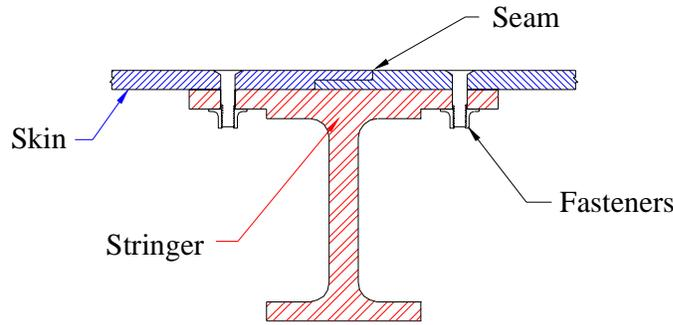
Figure 1: Aircraft Skin Assembly, Fasteners with Stringer.
