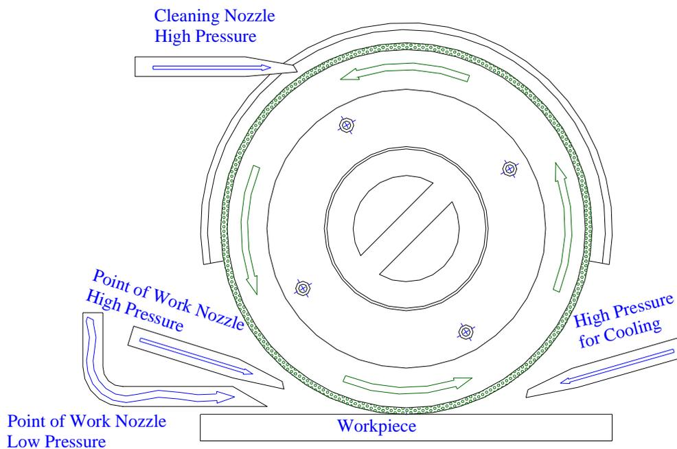
Figure 5: High Pressure Coolant System - Test Configuration
