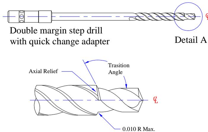
Figure 2: Typical Aircraft Drill, for Pre-drilling Fastener Holes.
