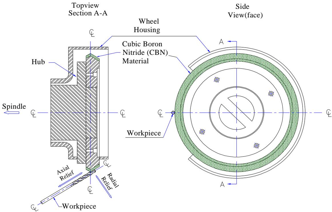
Figure 3: Workpiece and Wheel Configuration - Pilot Grinding Process for Step Drills
