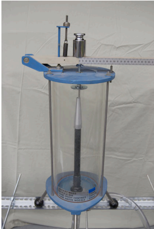
Figure 4: Laboratory apparatus for Virtual Lab #1 (manufactured by TecQuipment, Ltd.). The nozzle discharges a jet of water that impacts the deflector plate. A weight is used to balance the force of the impact jet, and moments are summed about the hinge to calculate the force due to the jet of water
