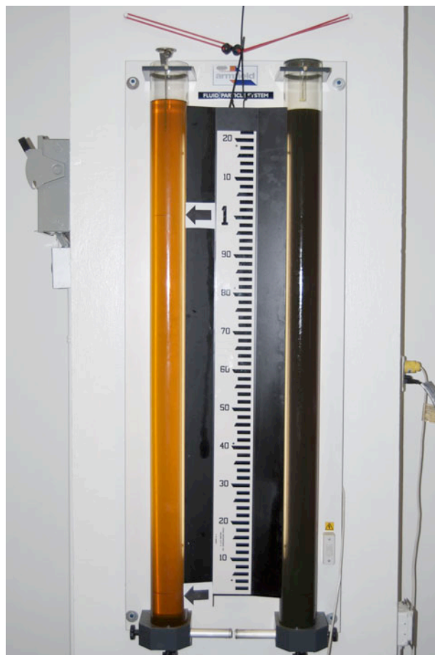
Figure 6: Apparatus used to determine the drag force on a sphere falling through columns of different fluid (by Armfield, Ltd.). SAE 50 (left) and NAPA 20 (right) oils were used for the experiment.
