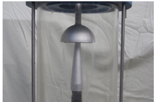
Figure 5: (top) Flat-plate deflector and (bottom) hemispherical deflector used for laboratory observations. The shape of the hemispherical deflector provides a theoretical 2-fold increase in the vertical component of force due to the water jet over the flat-plate deflector.
