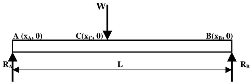
Figure 2. Reactions at the supports of a simply supported beam.
