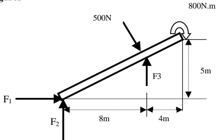
Figure 1. Neglecting the weight of the beam, find forces  $F_1$ ,  $F_2$ , and  $F_3$ .
