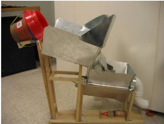
Fig. 5: Solution with spring lift, mechanical delay, hole sizes to separate. FoM=2.61; artifact 0.87.
