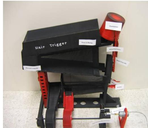
Fig. 6: Solution with spring lift, mechanical delay, holes sizes to separate. FoM=1.68; artifact=3.0.
