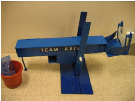
Fig. 1: Solution with gravity fulcrum lift, mechanical delay timer, and drop holes to separate. FoM = 2.86, artifact = 3.53.
