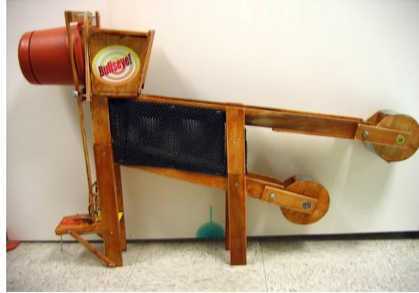
Fig. 4: Solution with spring lift, gravity driven oscillating timers, nearly parallel rods to separate. FoM =4.48; artifact 3.93.
