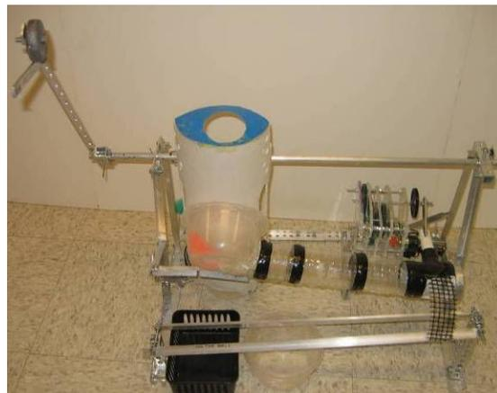
Fig. 2: Solution with gravity torque lift, motor-driven rotating aperture timer, nearly parallel rods to separate. FoM=3.94; artifact=3.67.
