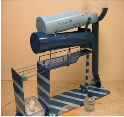
Fig 3: Solution with spring lift, mechanical Delay, nearly parallel rods to separate. FoM=3.53; artifact =2.87.
