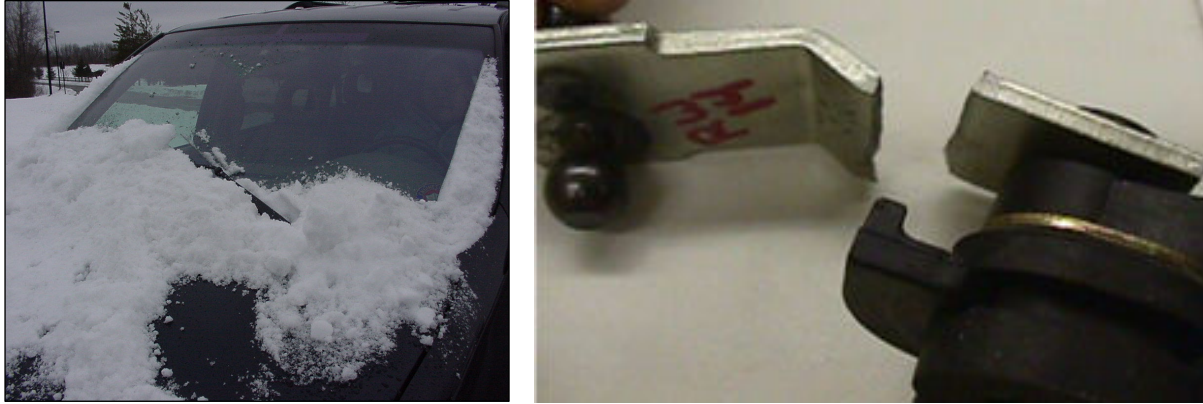
FIGURE 7 – WINDSHIELD WIPERS UNDER SNOW LOAD THAT BREAKS A ROCKER ARM
