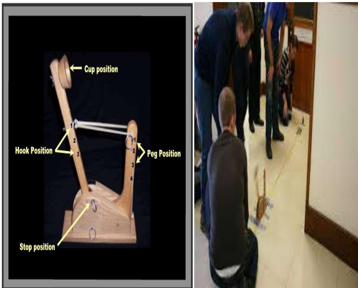
**Figure 3. (a)Image of a Statapult and its Components; (b) How it is Used to Launch a Ball**
