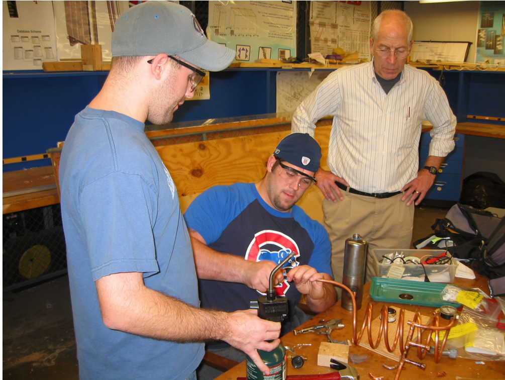
Figure 3. The water heat pipe assembly in progress.
