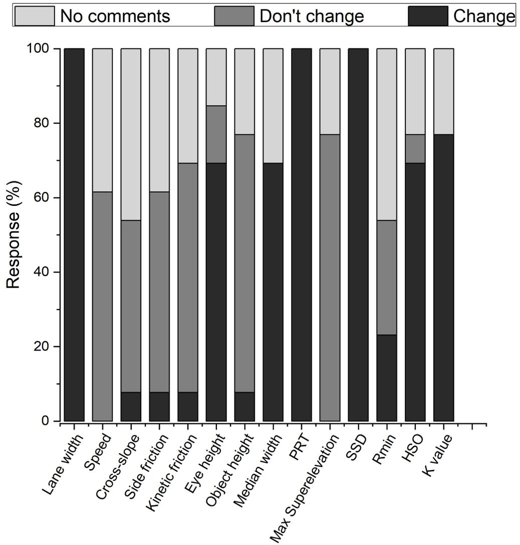
Figure 4: Modifications to geometric design criteria for AVs suggested by class project teams.
