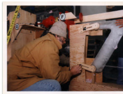
4—Mounting ice bridge for testing
