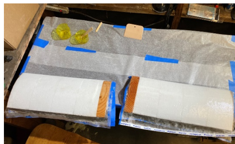
Fig. 10 Attached foam core segments
