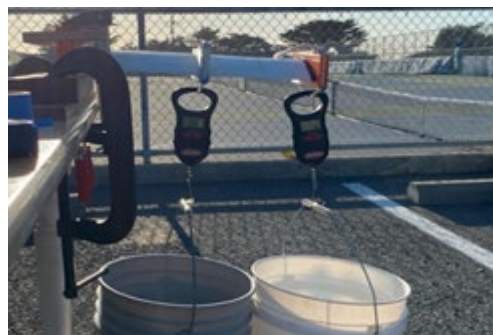
Fig. 11 Wing bending test setup
