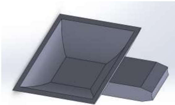
Figure 8a: One of the six identical pelton buckets.
