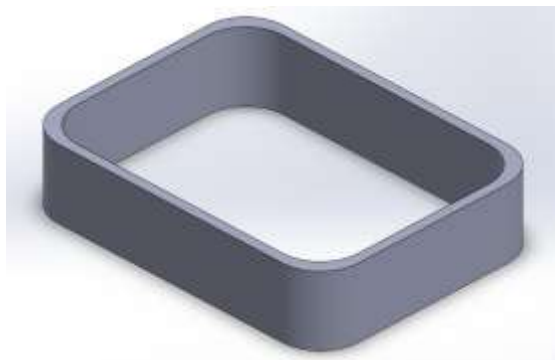
Figure 3: The bottom gutter attachment.
