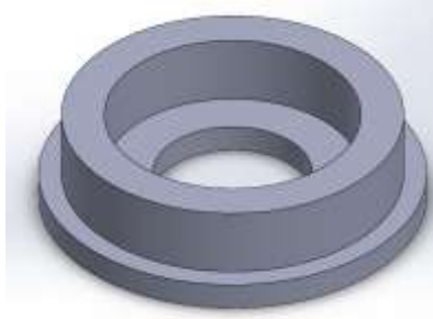
Figure 6a: The through-hole bearing attachment.
