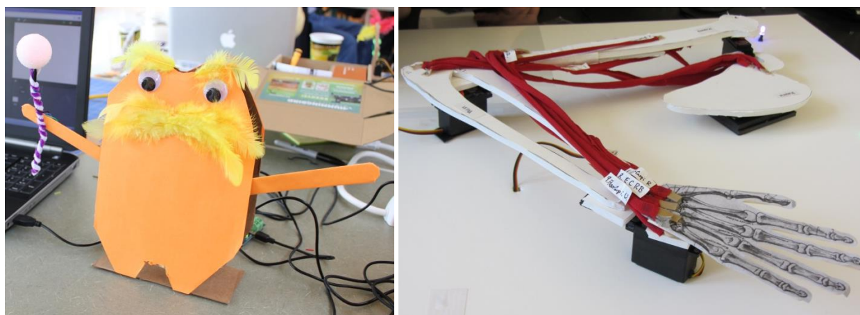
Figure 1. (Left) An Arts & Bots robot based on Dr. Seuss's poem The Lorax with servo motors to move the arms and an LED to light the "truffula tree". (Right) An Arts & Bots robot model of a human arm musculoskeletal system with servo motors to move the joints.
