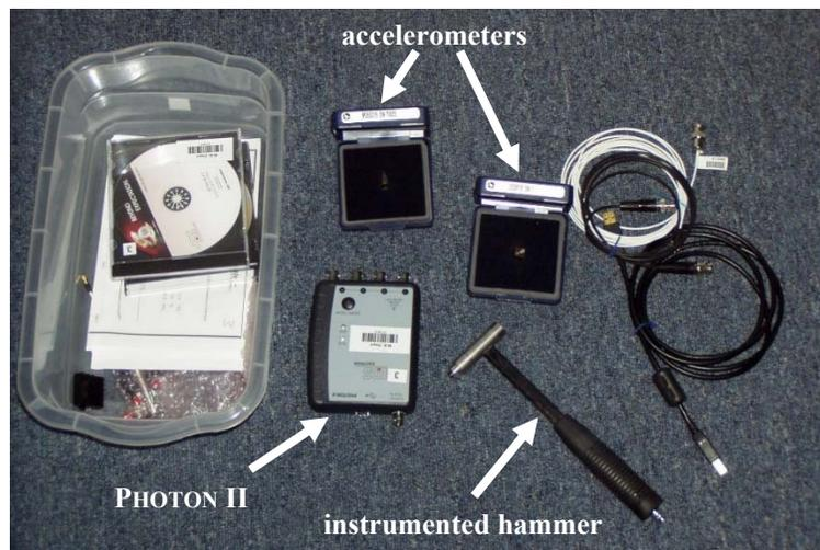
**Figure 1.** The contents of a vibrations kit used in the lab.
