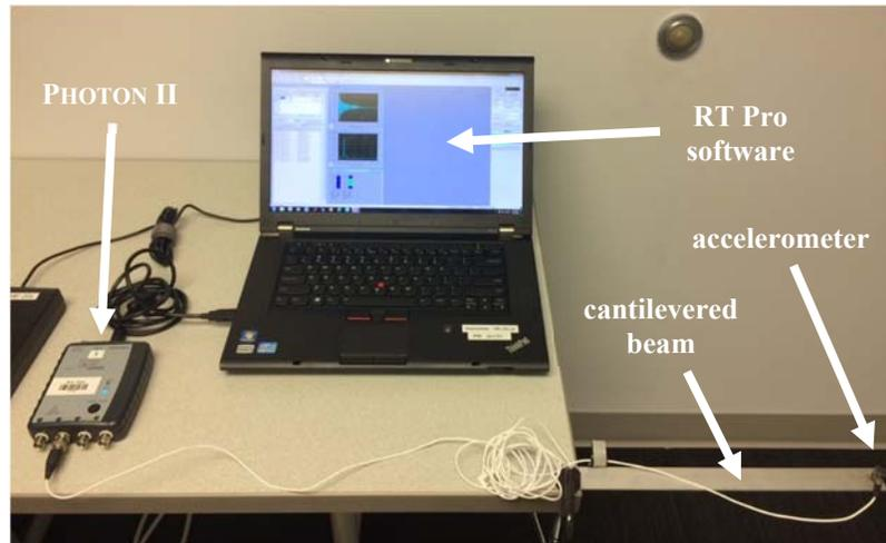
**Figure 2.** A PHOTON II device interfaced with a laptop running RT Pro to collect data for the cantilevered beam experiment.
