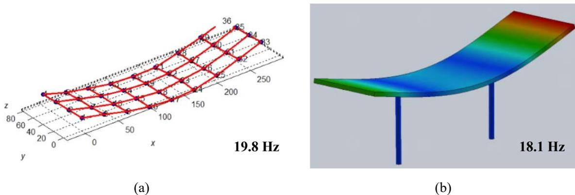
**Figure 5.** (a) Experimental results and (b) finite element results for the second mode of the lab table in Figure 4.
