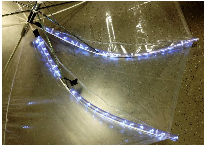
Figure 3. A prototype version of two LED light strings with the LEDs soldered into a parallel circuit and inserted into colored plastic tubing. The tubing is attached to the umbrella ribs by clear zip-ties.
