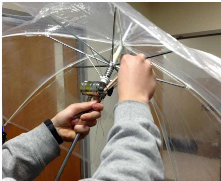
Figure 1. A second iteration of the “Illuminated Umbrella” power supply showing the DC motor attached to the umbrella axial runner and hand crank mechanism.
