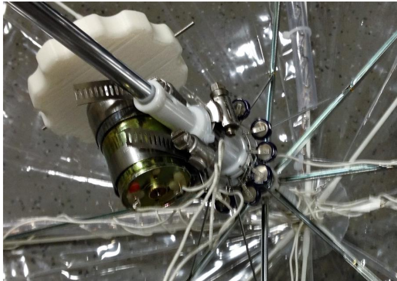
Figure 5. The final design arrangement of the “Illuminated Umbrella” DC-motor power-supply attached to the umbrella central runner, parallel circuit of 1/3 Farad capacitors (i.e., ring of dime-sized components around central shaft), and hand-wheel that replaced hand-crank. The clear plastic tubing containing the LED lights and zip-tied to the umbrella ribs is also visible in the background.
