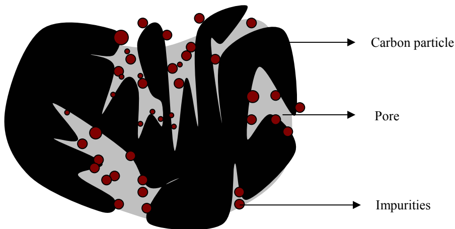
Fig. 1. Activated carbon granule shown with the adsorbed impurities
