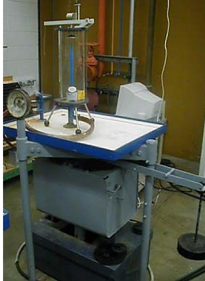
Figure 2: Physical Set-up of the Jet-force on Vanes Experiment.
