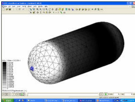
Such a tank is shown in Figures 13 and 14. In Figure 13 the tank is fixed on the side, so that the maximum radial deflection can be determined. In Figure 14 the tank is held from the end, so that the maximum longitudinal deflection can be determined. The results agreed well with the manually calculated results.
