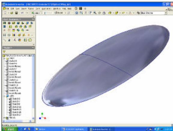
**Figure 20. Predator Virtual CNC Machining of Elliptical Wing**
