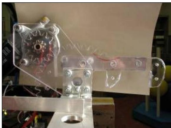
**Figure 6. Lexan Pinion on Ford Window Motor**
