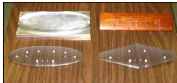
surfaces to hold on to. To solve this problem the students first machine a negative (which is shown in the upper left corner of Figure 21) and put in some tapped holes for tie down screws. Two holes are reamed for dowel pin insertion in order to provide for very accurate positioning. The students have been very happy with the quality of the wing models that they have been able to produce.
