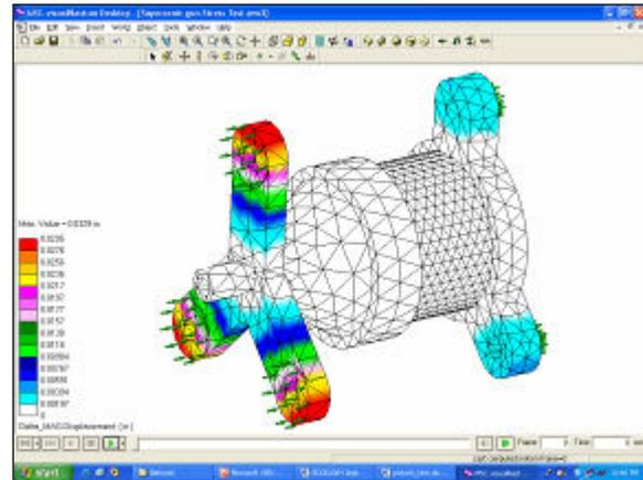
tripod for the assembly before the chamber could be pressurized. The simulation for the deflection caused by this preloading is shown in Figure 17. The students also calculated this deflection manually, after making some simplifying assumptions. Once the parts were
