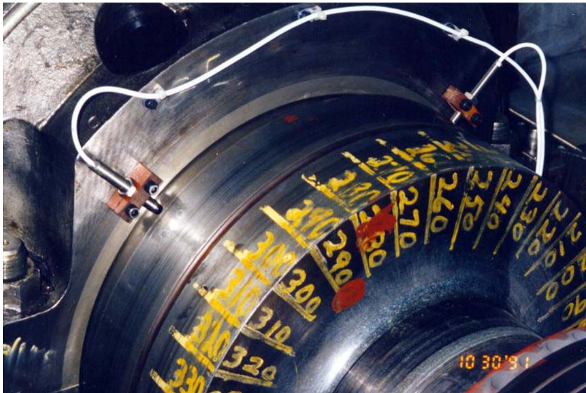
Figure 2: Close-up of the rotor showing the proximity probes
