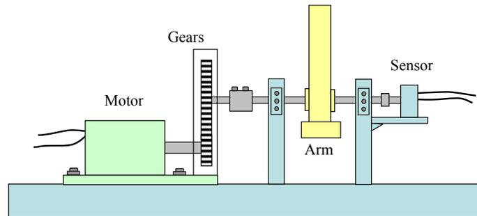
Figure 1: DC motor and arm setup
