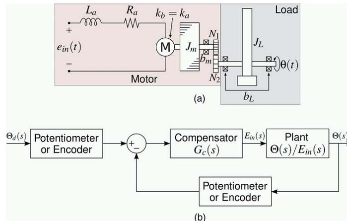
Figure 2: a) System schematic and b) Control system block diagram
