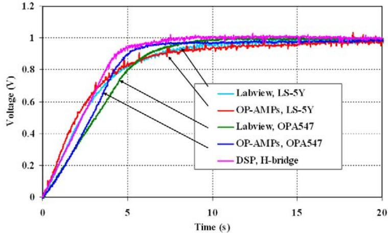
Figure 4: Experimental step responses of various PI position controllers
