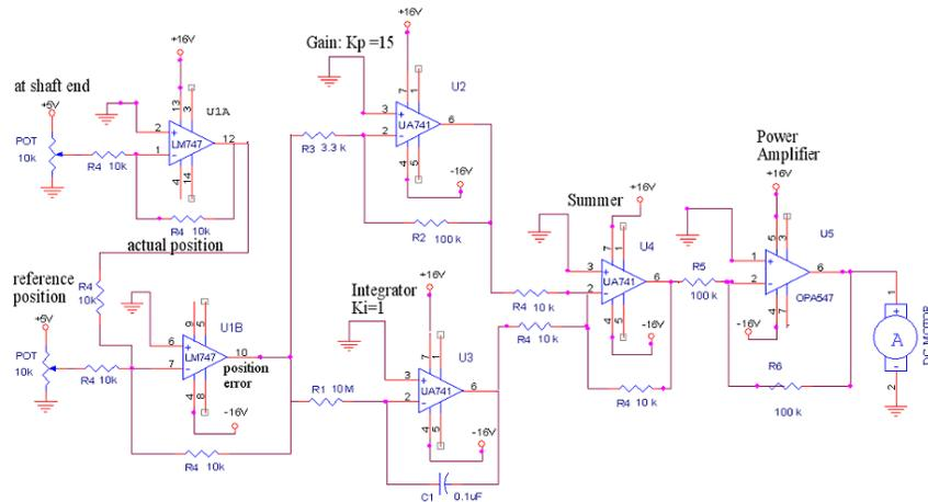
Figure 3: Implementation of an analog PI position controller using operational amplifiers
