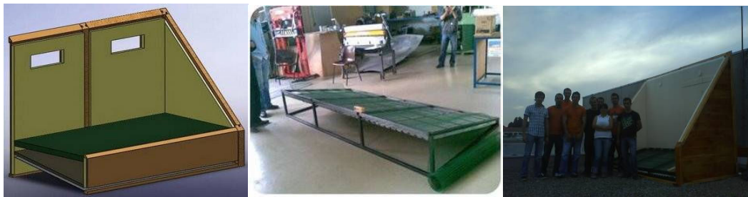
Figure 4. Solar kiln designed to dry 60 kg of local shrub species.
