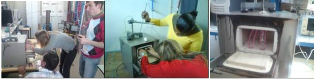
Figure 3. Wiring and preventing the thermocouple from direct exposure to radiation; IR emission.
