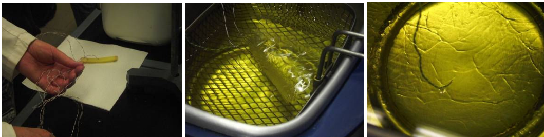
Figure 2. Wiring and frying the French fry (upper surface of a hot plate, natural convection).
