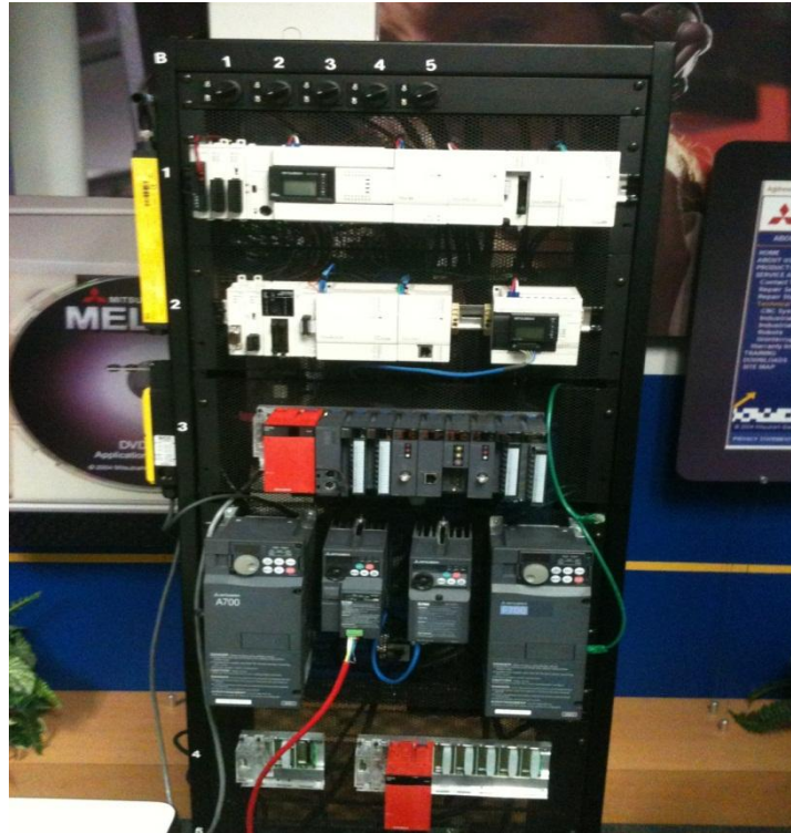
Figure-2 Trainer Rak with VFD and Servo Drivers
