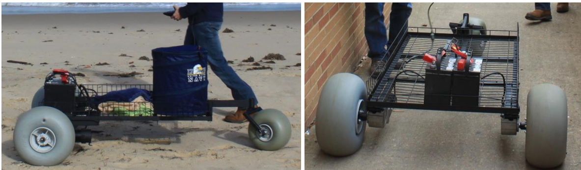
Figure 3: Multi-Surface Electric Cart tested on various surfaces 29
